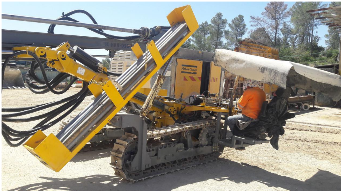
HAN-D50-DTH Pneumatic Crawler Drilling Rig in Middle East Borehole diameter: 90-165 mm
